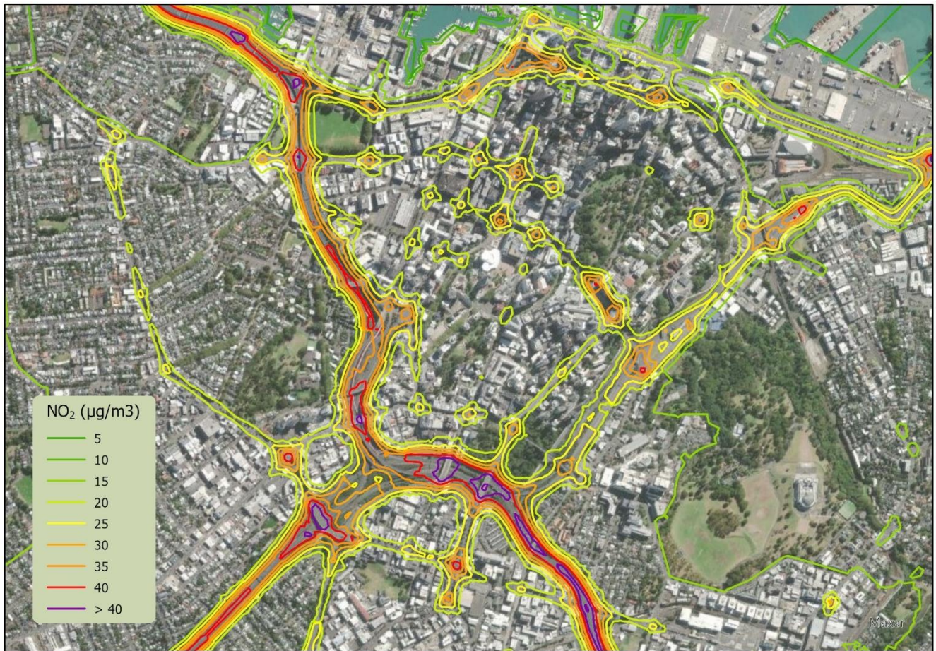
Figure 6.6: Example GIS output showing concentration contours of NO 2 in 5 µg/m 3 increments outputted from the VEMT and concentration calculator
